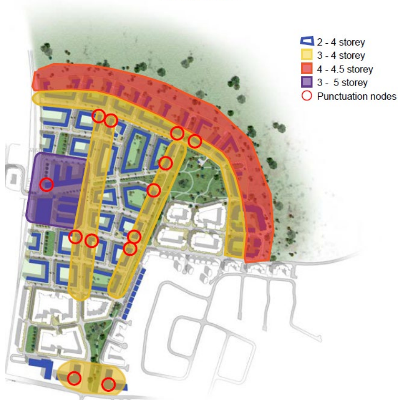
Figure 4D.2 Building Heights
